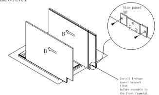
Step 3: Install bottom panel. Insert the bottom panel (C) into groove of side panel (B) until it into the groove of front frame (A).
