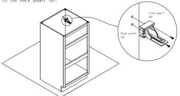
Step 10: Insert drawer slide runner to the rear slide bracket and screw the drawer side to the guide hole of front frame (A) and hole for drawer slide
