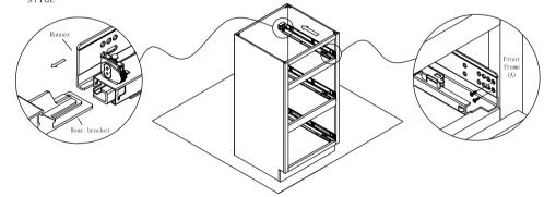
Step 11: Put the drawer box on the drawer slide and push the drawer box to make the end of runner is lock to the hole of the drawer back panel. Complete the installation of the drawer box when your hear sound click which mean the locking device is locked on the drawer slide.
